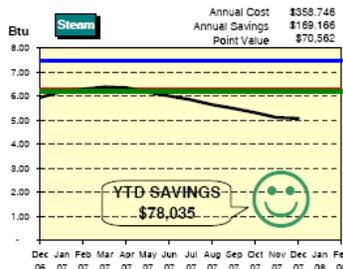
The Energard Index is annual energy use per square foot of conditioned space adjusted for changes in outside temperature (Degree Days). Each monthly value is a sum of the previous 365 days of use (rolling annual total). An Index trend down indicates savings; an Index trend up indicates loss. When the Index trend is below the Base Line, savings are generated. The Alert Set Point is 1% above Last Year Index. Base Year Index is presently: 2003
